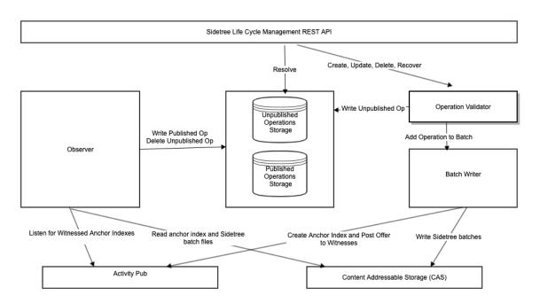
Orb node will validate each Sidetree operation as per specification. Valid operation will then be added to the batch writer queue and unpublished operations store. Batch writer will then batch multiple Sidetree operations together and store them in Sidetree batch files as per Sidetree file structure spec.
